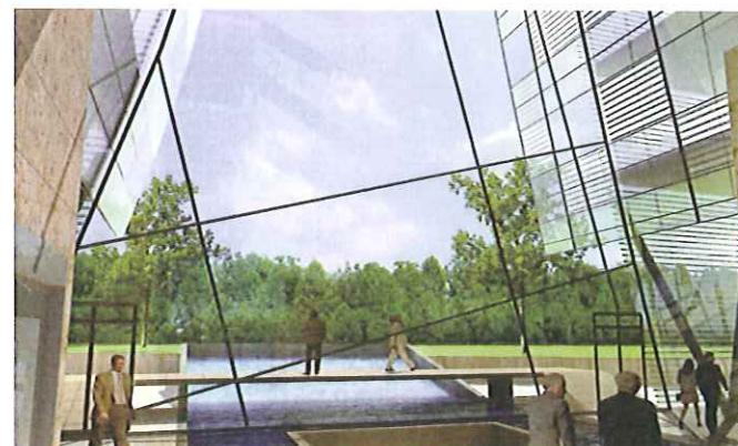
ing to achieve the desired outcome." Trevor Dillon, contracts manager for Tiber Bonvec Construction, says the glazed façades are made up of a unitised aluminium and glass system with components that slot into one another, and eliminate the need for excessive scaffolding.
